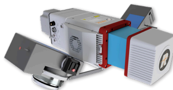
with two Sony Alpha 6000 cameras (oblique mount)
